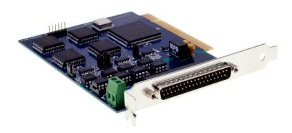
The PCI4 is a PCI 2.1 compatible PC expansion card that provides four channels of magnetostrictive linear transducer interface. When commanded by the host PC, the module interrogates the sensors and returns position data to the host PC. When operating with Start/Stop and PWM output sensors, the received pulse timing data is converted to position data and returned to the host PC. When operating with SSI output sensors, the received data word is made available to the host PC.
